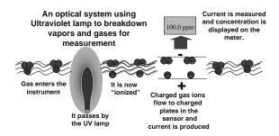
with a *detector*. The detector measures the charge of the ionized gas and converts the signal into current. The current is then amplified and displayed on the meter as "ppm." After measurement, the ions re-form the original gas or vapor. RAE PIDs are not dependent on oxygen to make a measurement and PIDs fail safe. When the PID lamp fails to light the PID provides a "lamp" alarm so operators immediately know that it is not working.
