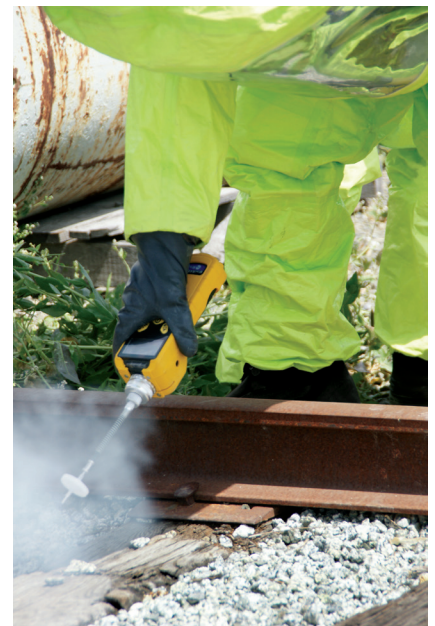
Workers can quickly measure VOCs and wirelessly transmit data via Bluetooth or optional Mesh radio.
